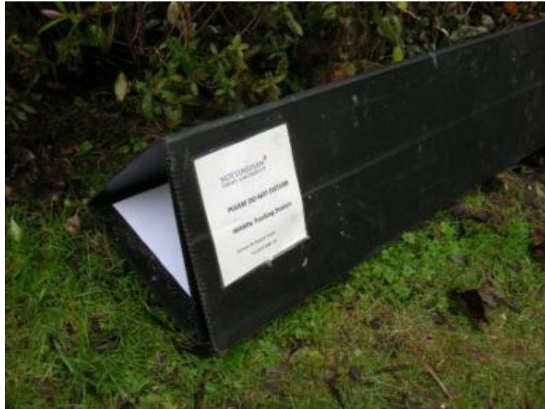
Fig. 2: A fully assembled hedgehog footprint tunnel, in place next to a hedgerow. (Photo: The Mammal Society).
